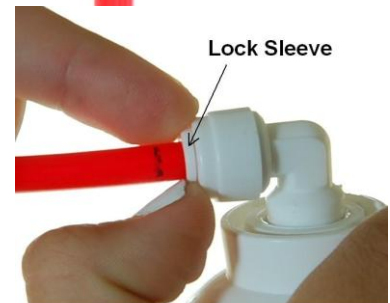
With two fingers PUSHING IN and PRESSING DOWN Lock Sleeve, pull out tubing
